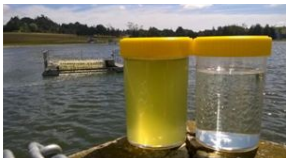
Wastewater at Wellsford, pre and post membrane filtration.
